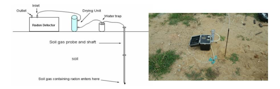
$\langle$  Measurement of Radon in soil gas  $\rangle$
