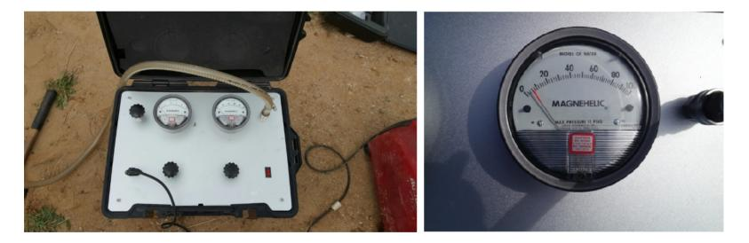
$\langle$  Measurement of air permeability in soil  $\rangle$
