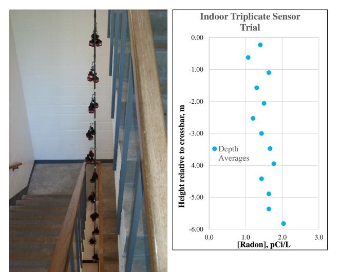
Figure (9): Indoor radon tower.
