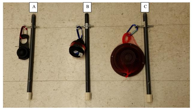
Figure (3): Suspending the E-PERM® sensors from the radon tower. A) L-OO chamber, B) S chamber, C) H chamber.
