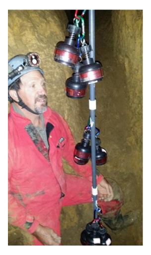
Figure (12): Kemling Cave internal radon tower construction.
